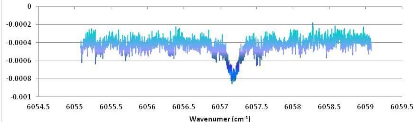
Example of 12ppm concentration of methane in 80cm flowcell. Simulated using HITRAN methane data and actual scanned cell data. Used Agilent 8164A tunable laser to scan line. 0.02% is roughly the noise floor of the laser.
